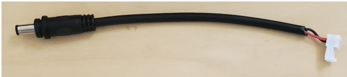
S0074-00103: Controller to Display Power
