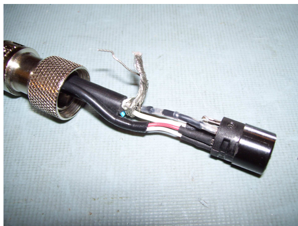
Re-solder the black wire to pin 7
