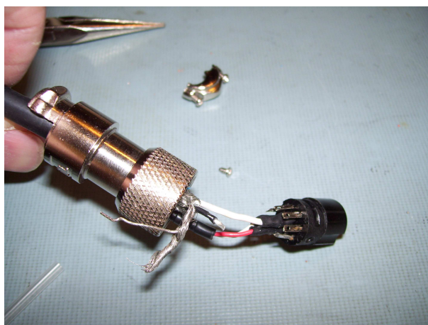
Slide the shell & plastic ring away from the 8-pin connector
