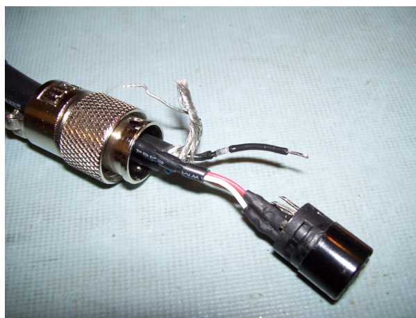
Unsolder pin 7 from the connector and cut the shield wire off of it
